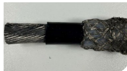
4/0 AWG cable 21mm OD semi-conductive layer insulation processed with the Mercury 6
