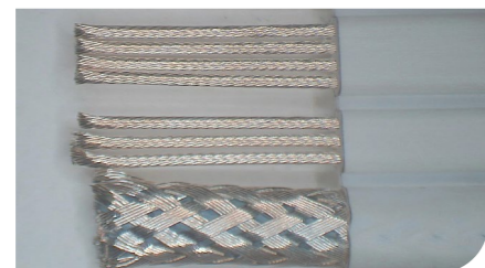
Flat cable, 41mm wide with 11 conductors connected together processed using the Mercury 4
